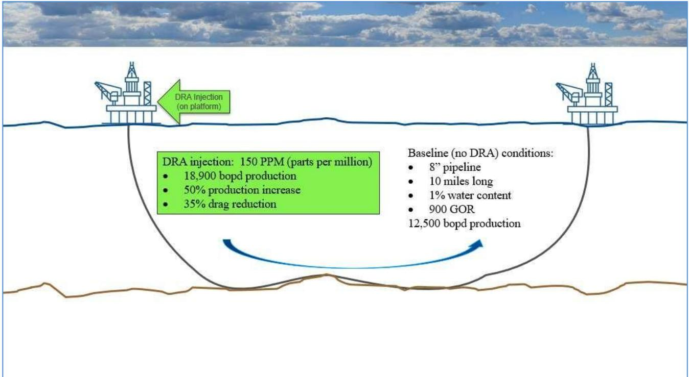
Figure 2, Platform-to-platform multiphase application case study
