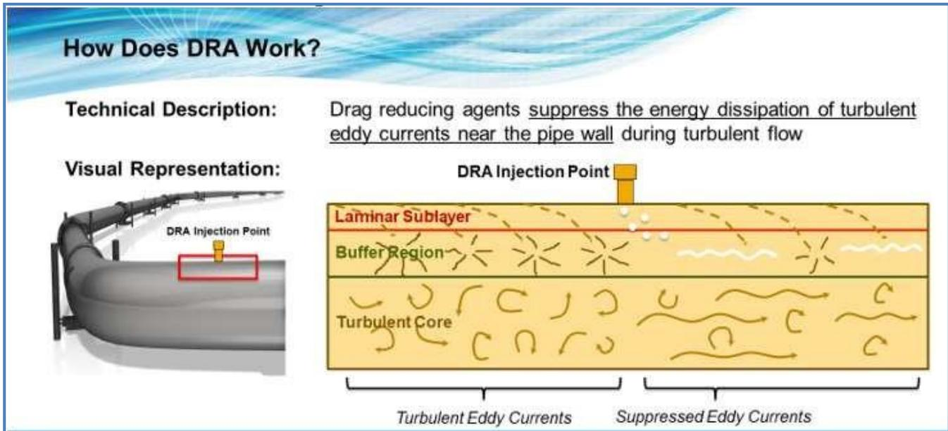
Figure 1, DRA suppresses turbulence, reducing frictional pressure loss along the flowline
