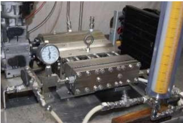
Figure 15, Modified triplex injection pump
