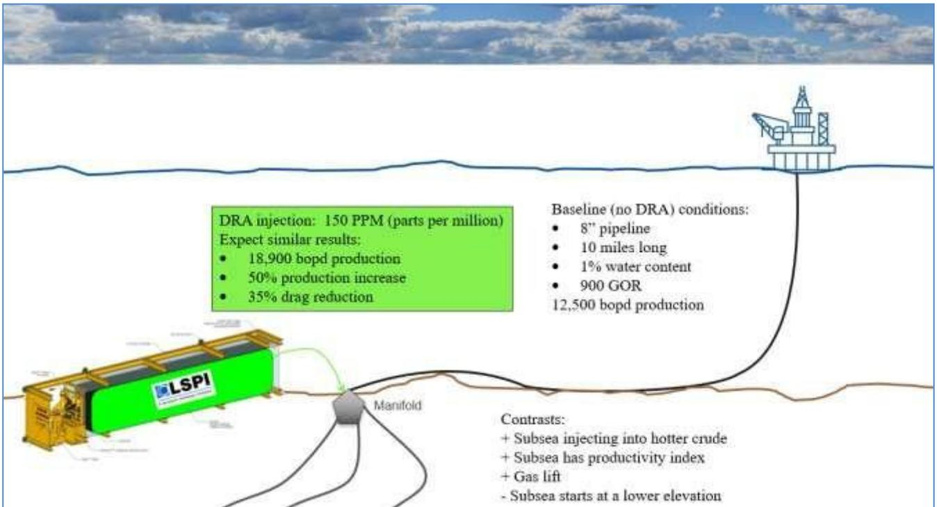
Figure 3, Extrapolated subsea DRA injection
