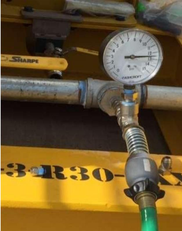
Figure 19, Steel tank pressure testing
